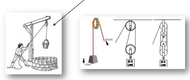
By using more than one pulley you can create a mechanical advantage. The more pulleys you use, the greater that advantage is. Diagram shows a pulley system with a mechanical advantage of 2:1. It allows a load to be raised using only half the effort needed using a single pulley, but twice as much rope must be pulled in.
